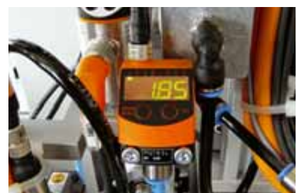
Pressure measurement in pneumatic systems.
